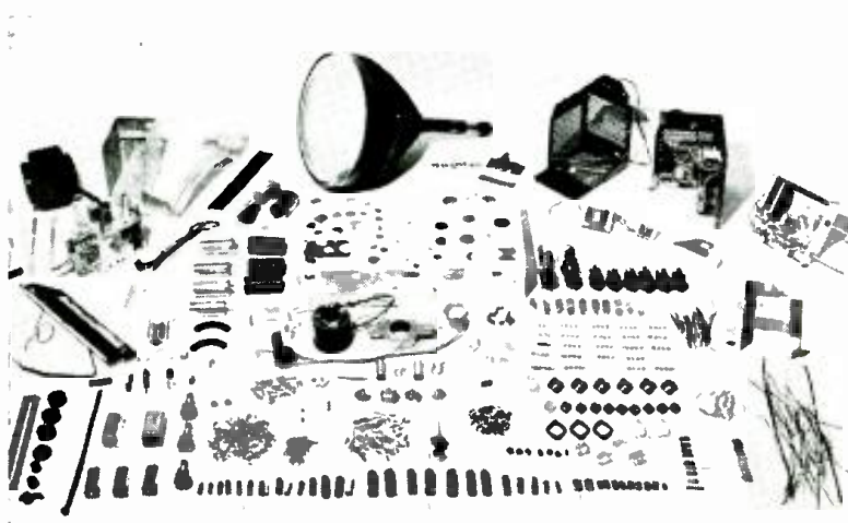
Figure 1 Layout of parts normally used in a layer-built chassis, using a 12 \frac{1}{2} " tube. Required are about 1,100 parts and components individually mounted, requiring about 500 solder connections.
