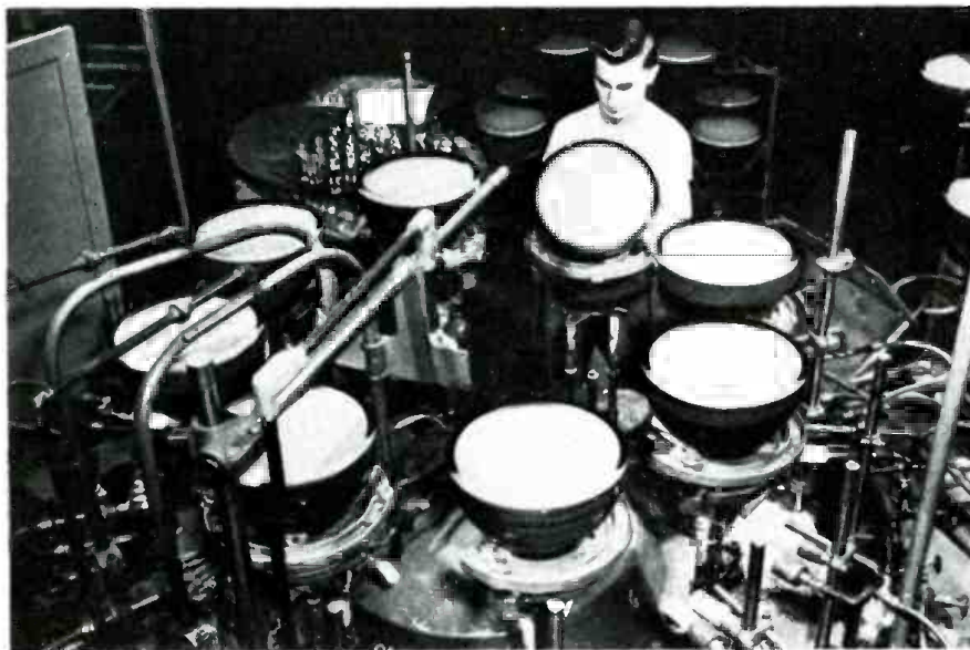
TV picture tube production at the Ottawa, Ohio, plant of Sylvania. At left, removing an assembled tube, which is ready for automatic exhaust and processing.
