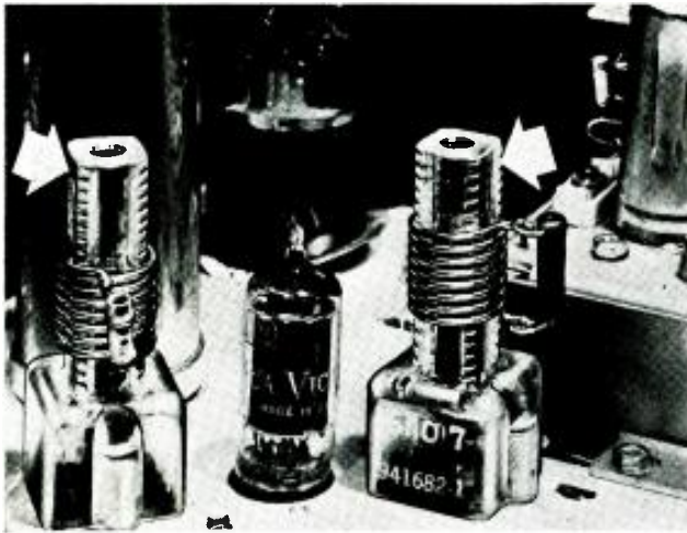
IF transformers with polystyrene coil forms which are said to help provide less rf losses and consequent improved rf gain. Tests have also revealed that the use of the polystyrene forms provides higher attenuation or selectivity of the if trap circuits, an improved performance which was found to eliminate one if trap circuit in a model.
