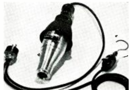
Below: The video analyzer used in predetermining of lighting.
