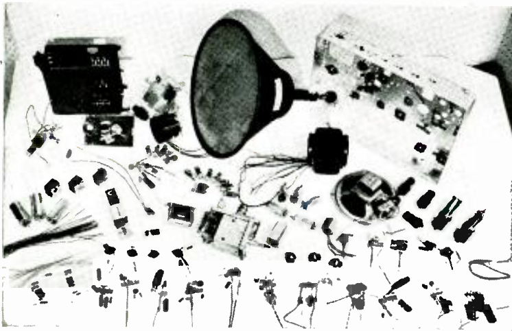
Prefabricated units developed for new streamlined chassis, which have 30 per cent fewer parts and 20 per cent fewer connections.
