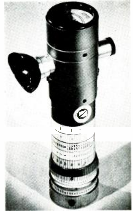
Right: Recently developed exposure photometer.
